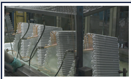
AIR UNDER WATER TESTING
